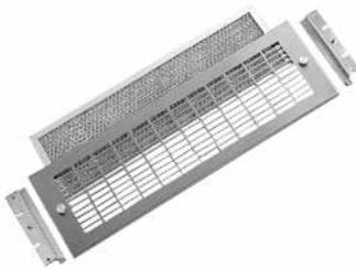
Located at air discharge side of an enclosure using Blower Package ADB275. Polished stainless steel grille is 65 percent open and offers low resistance to airflow. Expanded aluminum filter (included with each grille) is easily removed for cleaning from outside the enclosure. Mounting hardware is furnished.
