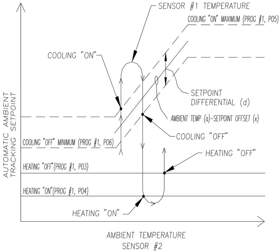
$$\begin{aligned} \text{COOLING "ON" SETPOINT} &= \text{AMBIENT TEMP} - X + d/2 \\ \text{COOLING "OFF" SETPOINT} &= \text{AMBIENT TEMP} - X - d/2 \end{aligned}$$
